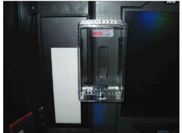
Figure 8.2 – Showing PEB slot covered with integral keyed locked enclosure.
