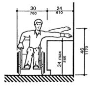
(17) The highest operable part of controls, dispensers, receptacles, and other operable equipment shall be placed within at least one of the reach ranges outlined in paragraphs (15) and (16) of this subsection.
