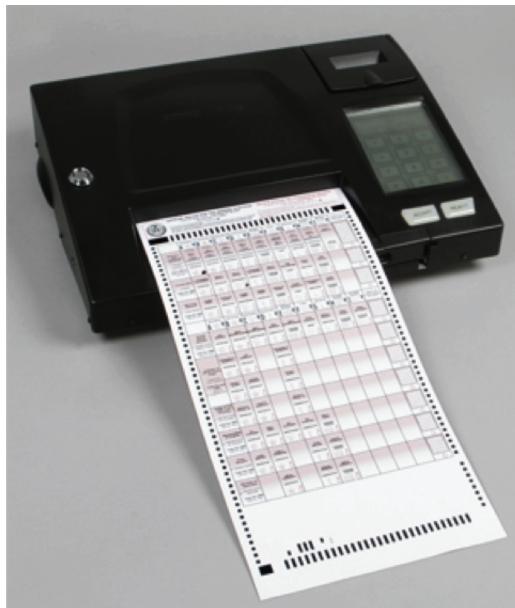
Figure 2-4: The ImageCast ® Precinct Ballot Counter
