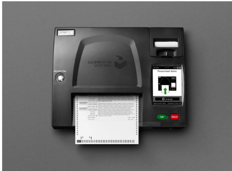
Figure 2-5: ImageCast® Precinct 2 Ballot Counter
