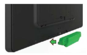
Gently insert the bar code scanner into the peripheral bay taking care to ensure the connector mates properly.
