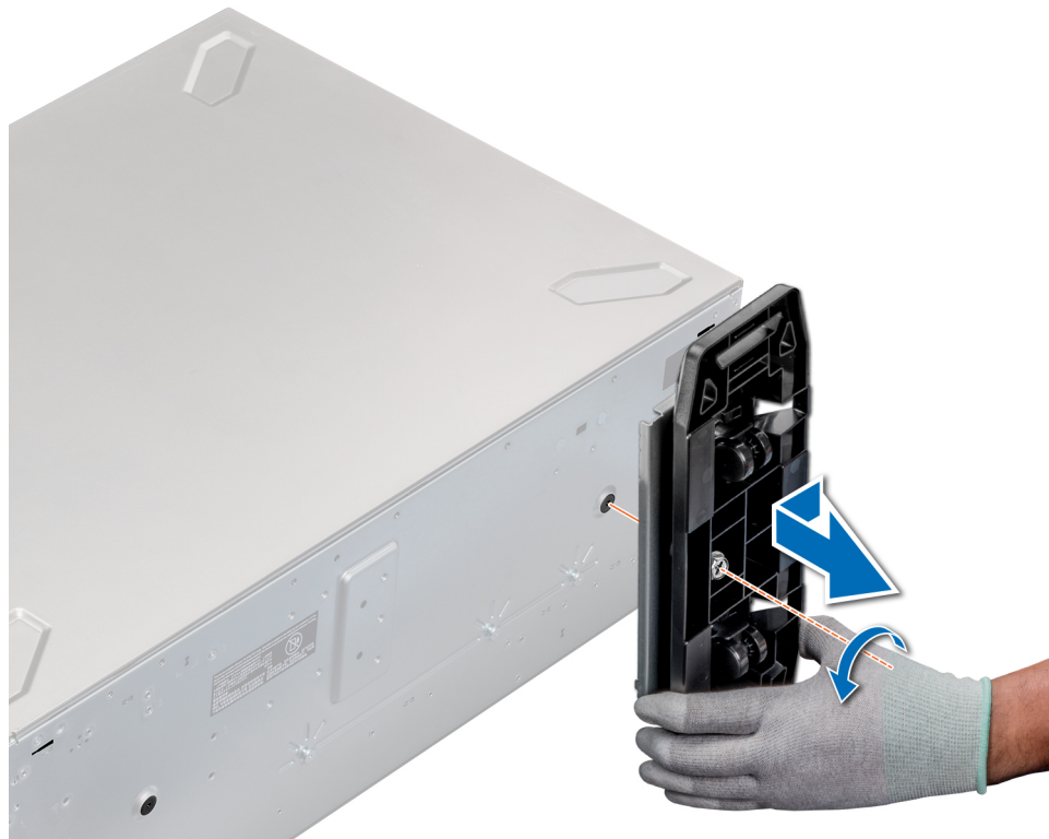
Figure 17. Removing caster wheels
