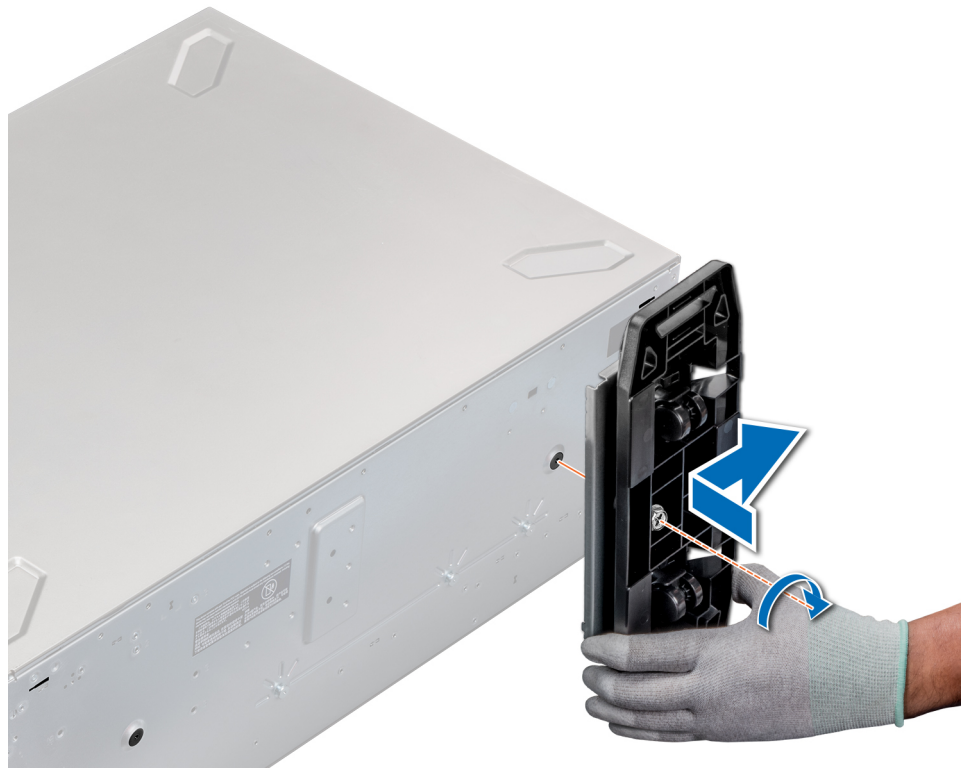
Figure 18. Installing castor wheels
