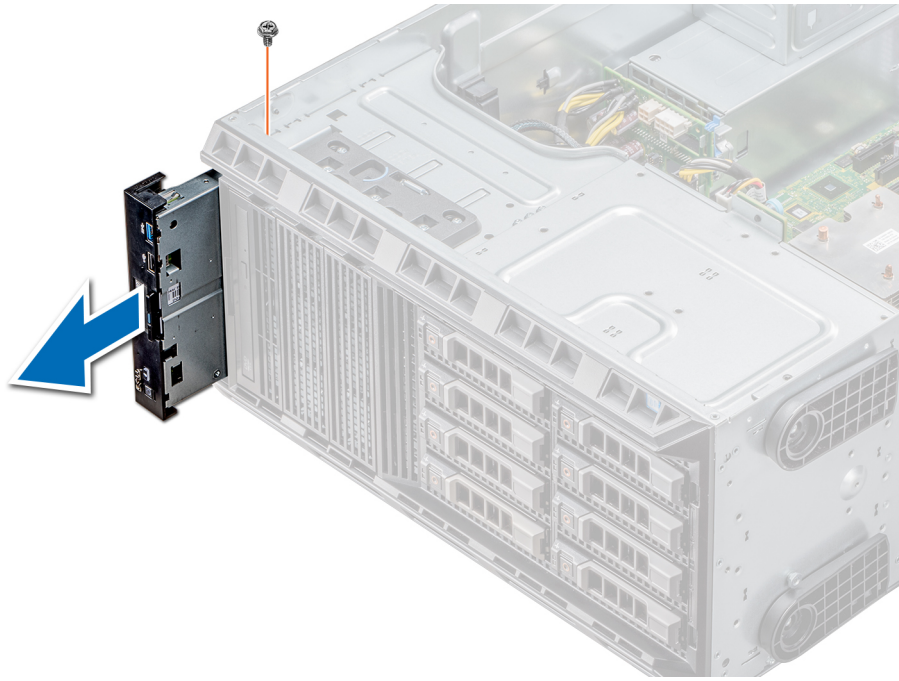
Figure 81. Removing the control panel assembly
