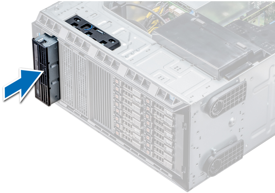
Figure 36. Installing the optical drive cage or tape drive
