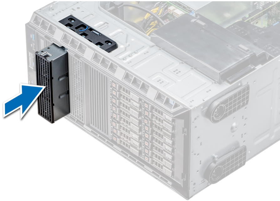
Figure 34. Installing the optical or tape drive blank
