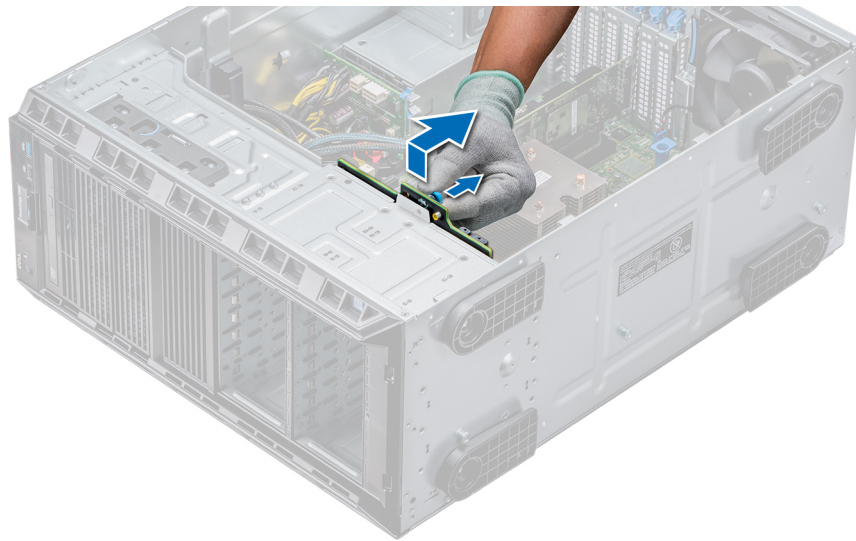
Figure 43. Removing a backplane
