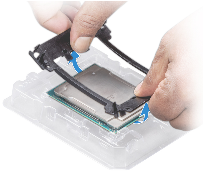
Figure 44. Removing the processor bracket
