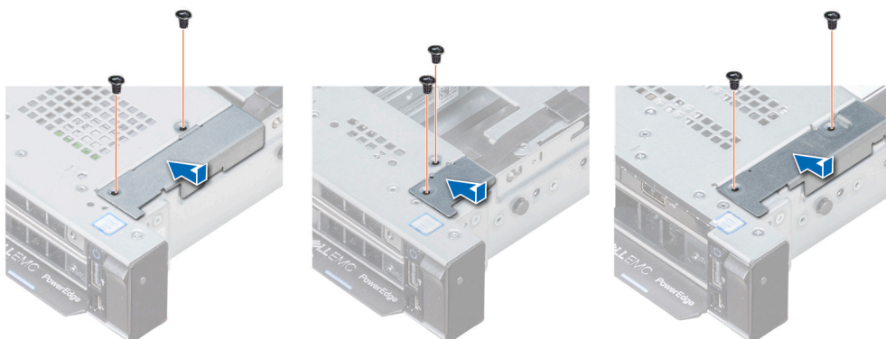
Figure 111. Installing the cable cover
