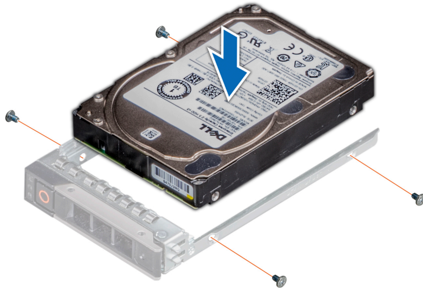
Figure 38. Installing a drive into the drive carrier
