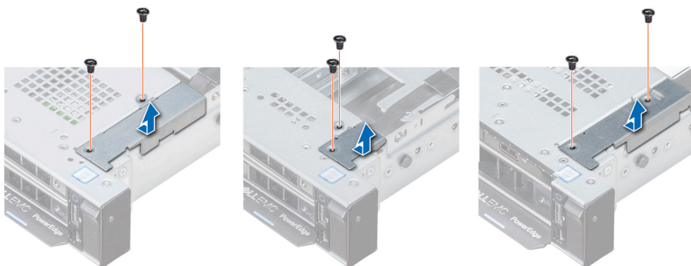
Figure 109. Removing the cable cover
