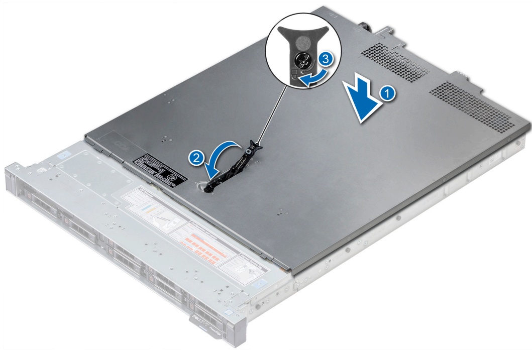
Figure 19. Installing the system cover
