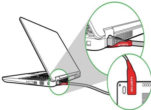
**Figure 4-1. A tamper-evident seal attached to an Ethernet cable connection**
