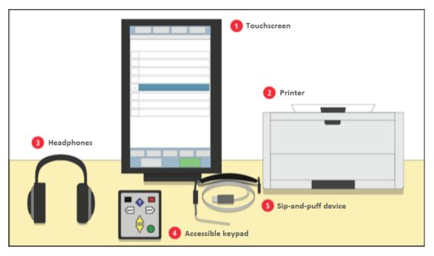
Figure 1-1. Hardware components of a ClearAccess system
