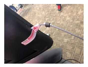
2. If the ClearAccess all-in-one is not connected to the ATI, apply a seal over the opening in bottom of the bezel that covers the opening entirely. Record the seal number.
